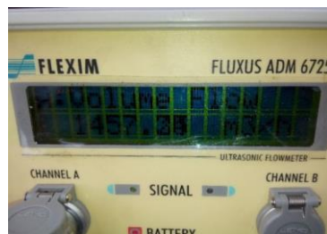
Fig. 5. Ultrasonic flowmeter recording a flow rate of 1457,33 m 3 /h.
