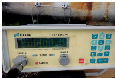
Fig. 3. Ultrasonic flowmeter recording a flow rate of 1449,90 m 3 /h
