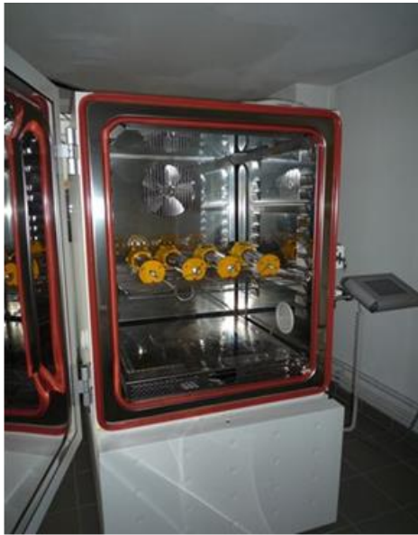
Fig.2. Lamps subjected to thermal endurance tests
