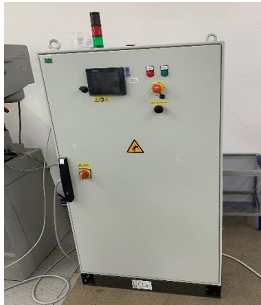
Fig.2. High voltage source Sefelec used to test the insulation systems of electric motor
